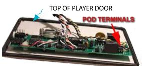
TURN POWER (circuit breaker) OFF and remove the 5 digital door screws. Tilt the door forward until you can access the back BOTTOM of the Player board.
